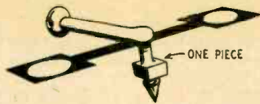
Fig. 5—Moving parts of tuned-ribbon pickup.
